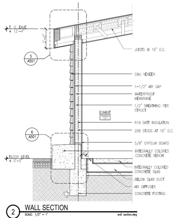
Using the architectural drawings set determine net wall area (sq. ft.) for each assembly ID using a scale and drawing take-offs. Gross wall area is the total wall area including fenestration; Do not subtract window area.
