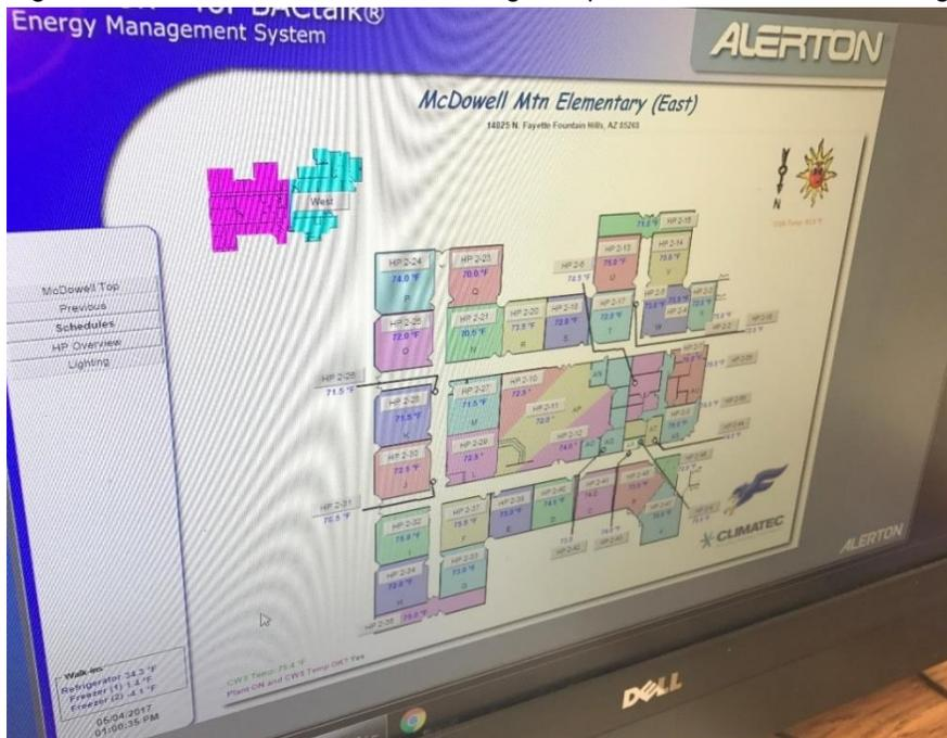
Figure 6018.5 BAS Screenshot Showing Temperature Setpoints for Each HVAC Unit
